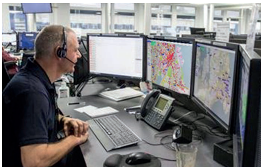
Greater Copenhagen has a register of 4,500 AEDs in Greater Copenhagen. The location of any AED less than 180 seconds transport from the site of call automatically comes up on the dispatcher screen (red dots in middle screen).
